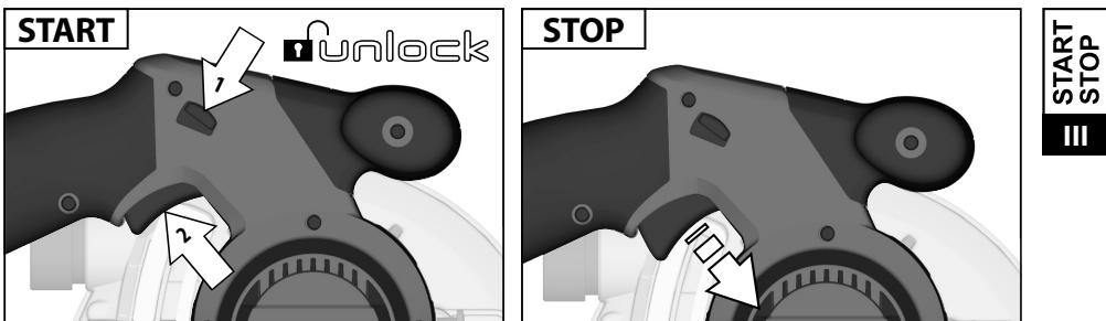
For safety reasons this power tool is fitted with a switch lock and the On-/Off switch cannot be locked in the "On" position
