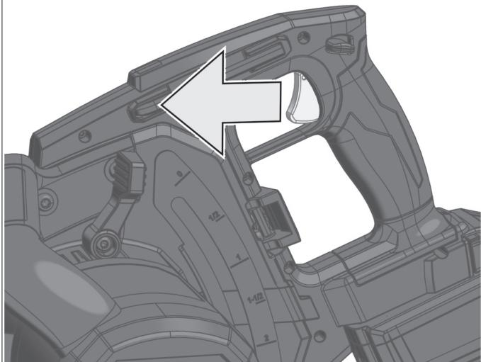
For safety reasons, the product is fitted with a switch lock, and the On/Off switch cannot be locked in the "ON" position.
