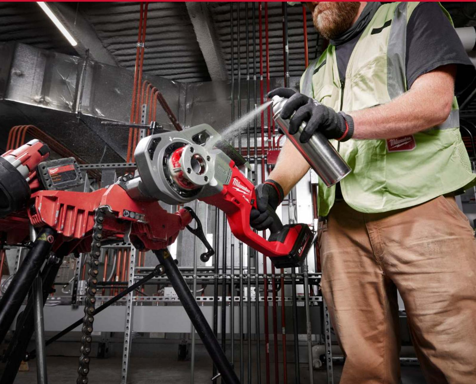
**M18 FUEL 1/4" COMPACT PIPE THREADER WITH 1/2"-1 1/4" COMPACT BSPT HIGH SPEED DIE HEADS M18 FPT114 ACCESSORIES**
